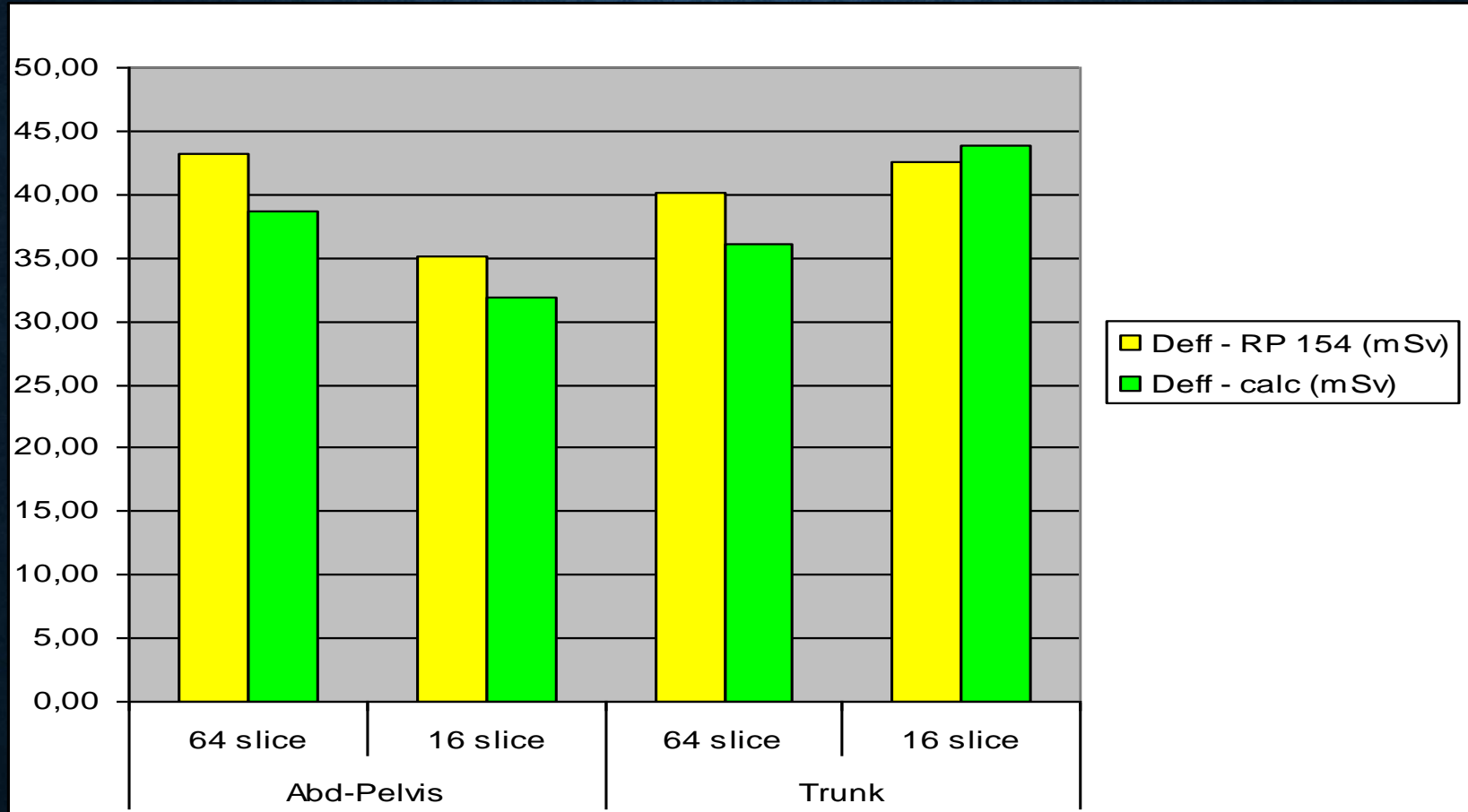
Fig.3 Effective dose (mSv) for 64 slice and 16 slice CT equipment, for AP and CAP procedures.
